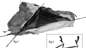
Start at the rear of the tent and insert the post end of the poles into the web grommets. See fig.2.
